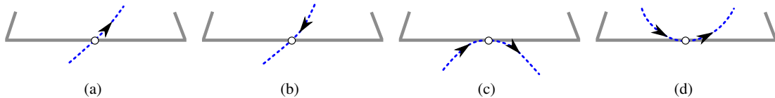
Fig. 2 Based on the flow at a point on the boundary of a triangle, the point can be classified as one of the following: (a) Inflow Point, (b) Outflow Point, (c) External Transition Point (ETP), and (d) Internal Transition Point (ITP).
