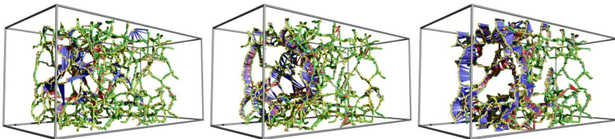
Figure 6: Tracking core structures between time-steps 500 and 12750 (left), 12750 and 25500 (middle), 5500 and 51000 (right). Red and blue lines indicate regions of greater displacement.
